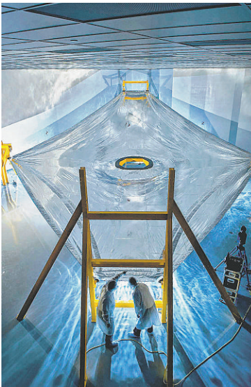
A sunshield membrane for the Webb Space Telescope is tested. PHOTO COURTESY OF NORTHROP GRUMMAN AEROSPACE SYSTEMS
